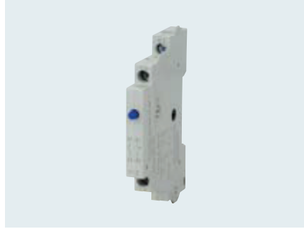
3VU9131-7AA00 S/C Trip indicating contacts 1NO + 1NC
